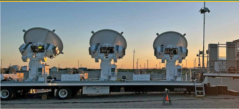
The U.S. Army Space and Missile Defense Command's Technical Center deploys the Spatially Enhanced Communications Tracking Reconnaissance and Engagements, a transportable distributed aperture research portfolio system, to White Sands Missile Range, New Mexico, in August 2024 to support a science and technology experiment. This transportable multifunction, multimission research system is presented in the trailer configuration. (U.S. Army photo)
