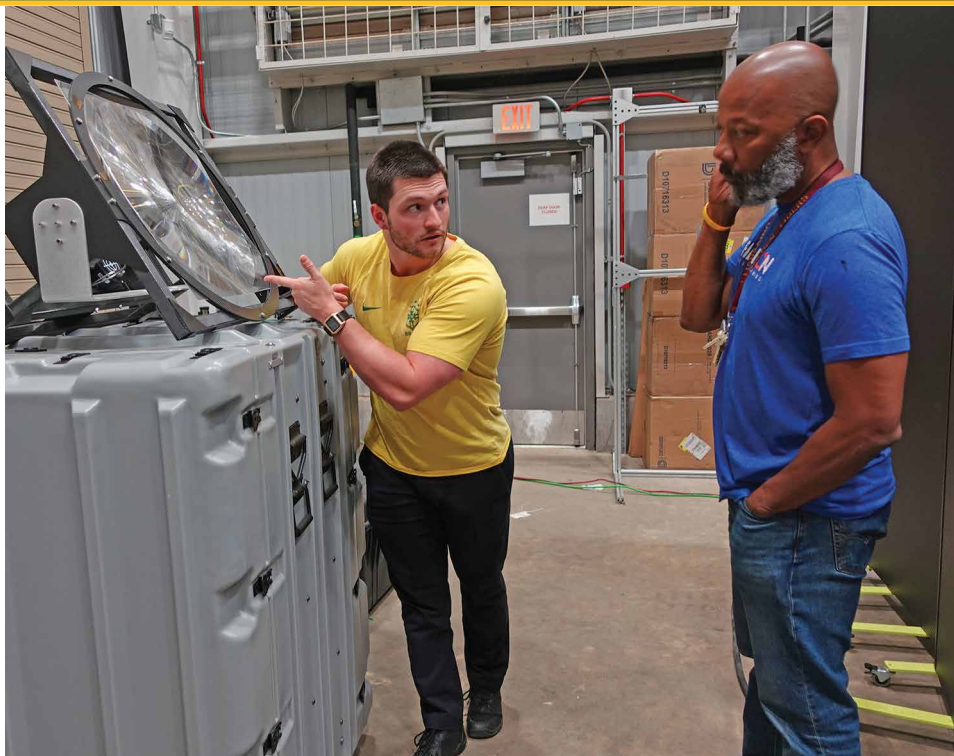
Cody Eberly, lab manager, Directed Energy Systems Integration Lab, teaches Steven Cephus about the Fresnel lens used in Big Aperture Shack-Hartmann – High Power, and explains plans to improve the system and mitigate light losses with the lens. (U.S. Army photo)
