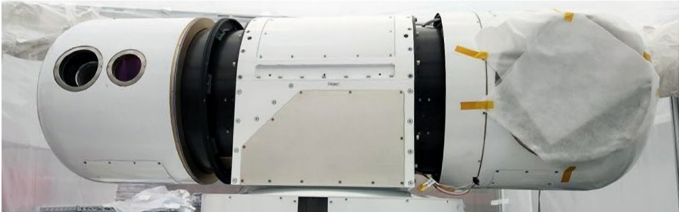
The Technical Center tests and evaluates the Affordable Laser Weapon Module for use in countering small unmanned aircraft systems in August 2022. (U.S. Army photo)
