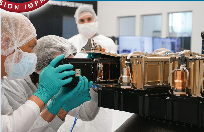
Members of the Gunsmoke program team place a Gunsmoke-J, a U.S. Army Space and Missile Defense Command and Assured Position Navigation and Timing/Space Cross Functional Team joint capability technology demonstration satellite, aboard a launch deployment vehicle prior to its June 30 air-launch from the Mojave Desert in California. (U.S. Army photo)
