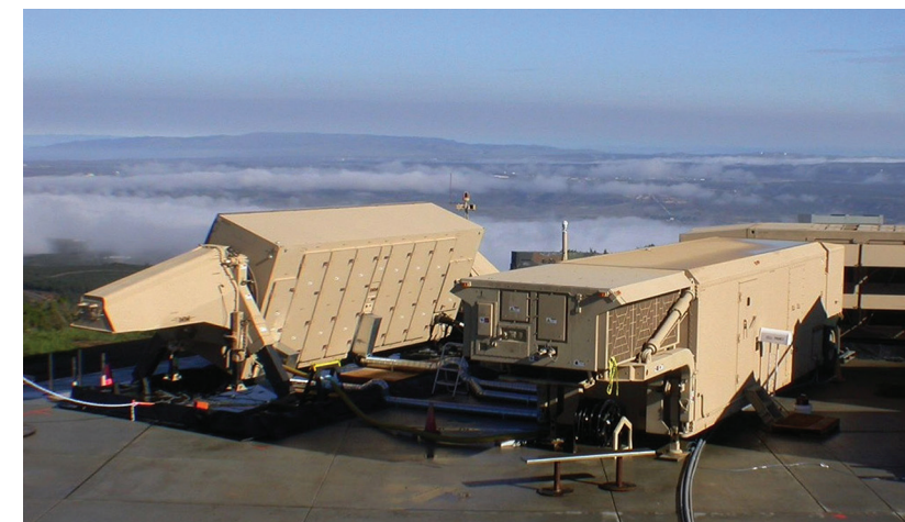
1 st Space Brigade batteries operate the AN/TPY-2, a missile-defense radar that can detect, classify and track ballistic missiles, in several locations around the world. (U.S. Army photo)
