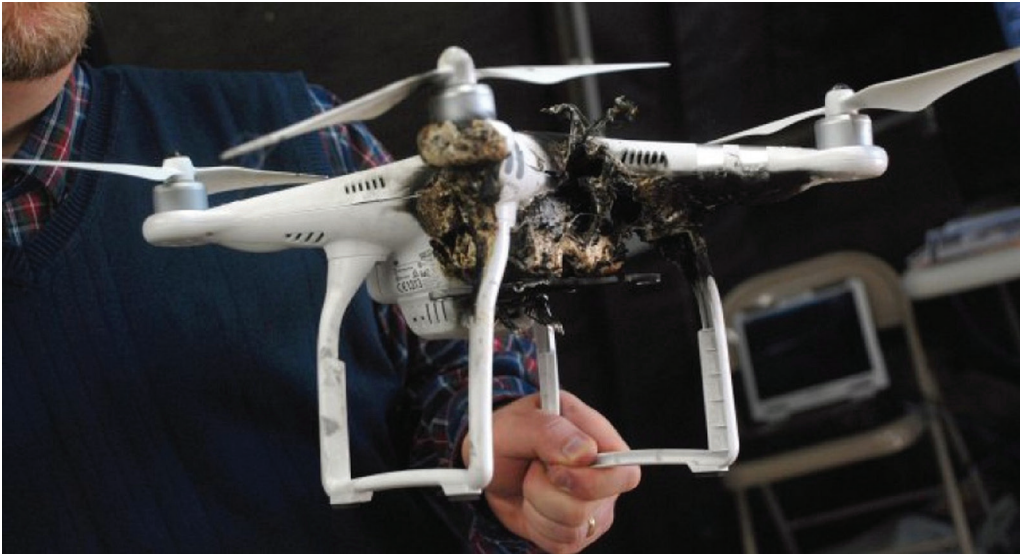
Adam Aberle, Directed Energy Directorate, Technical Center, holds an unmanned aerial system displaying the damage caused by a laser weapons system. (U.S. Army photo by Monica K. Guthrie)
