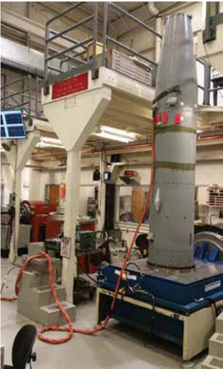
Black Dagger Target undergoes vibration testing at the NASA Wallops Flight Facility in Wallops, Virginia, in 2018, in support of the Black Dagger Risk Reduction Flight. (U.S. Army photo)
