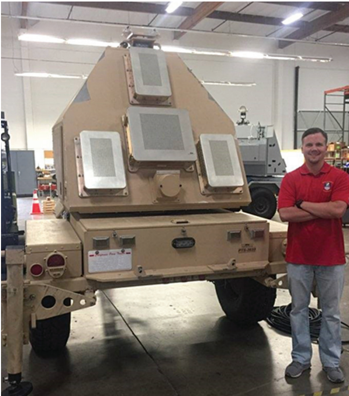
Jordan Dupree is the Concepts Analysis Laboratory’s technical lead for the Precision Track and Search Radar, which provides truth data for the counter-rocket, artillery and mortar, and counter-unmanned aerial system testing at Yuma Proving Ground, Arizona. The PTS system is operated by the CAL’s Science, Mathematics and Research for Transformation students/graduates, who also perform all mission planning and data analysis. (U.S. Army photo)
