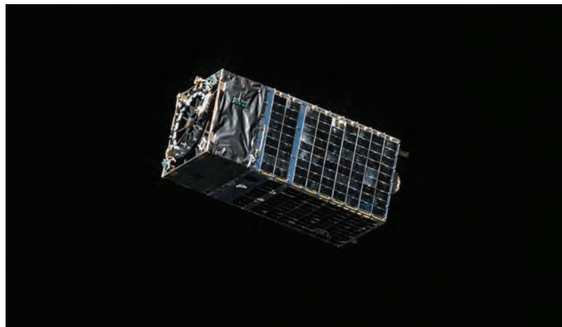
U.S. Army Space and Missile Defense Command/Army Forces Strategic Command's Kestrel Eye, a small, low-cost, visible-imagery microsatellite designed to provide near real-time images to the tactical-level ground Soldier, is a small business success story. Kestrel Eye was developed by a small business and its small business subcontractor.
