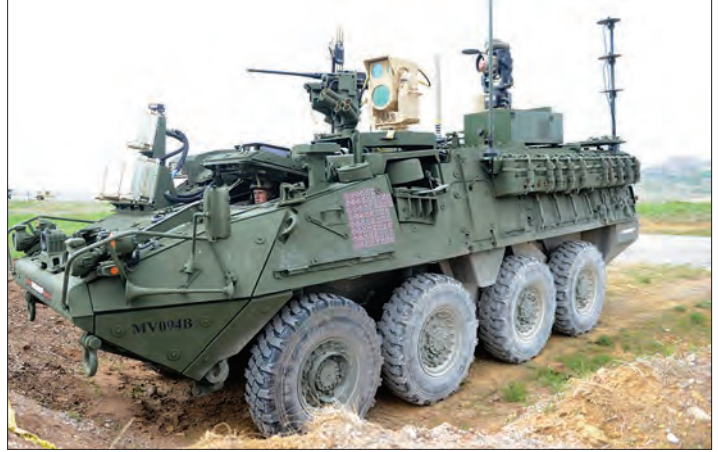
Mobile Expeditionary High Energy Laser is a laser testbed on a Stryker armored fighting vehicle chassis and serves as a platform for research and development.
