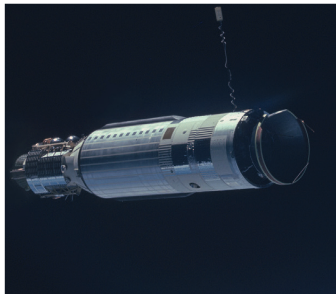
An Agena D booster stage photographed in orbit. One of these booster stages was the first successful satellite intercept scored by the U.S. at Kwajalein. 📷 NASA
