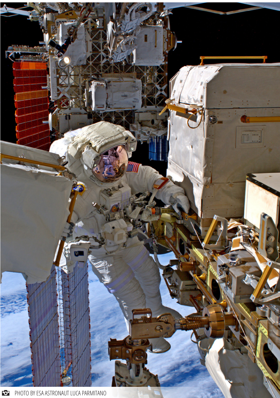
NASA astronaut U.S. Army Col. Andrew Morgan holds a new cooling module for the International Space Station’s Alpha Magnet Spectrometer during extravehicular activity #61, Dec. 2, 2019. Morgan worked with Italian Air Force and European Space Agency astronaut Italian Air Force Col. Luca Parmitano on this third of a series of four EVAs to repair the failing AMS, a state-of-the-art particle physics detector.
