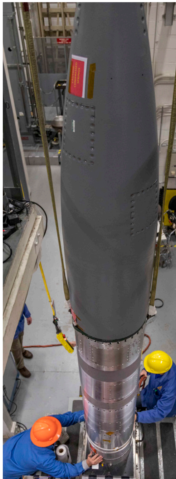
One of the two Too-WINDY payloads is prepared for vibration testing at NASA's Wallops Flight Facility prior to shipment to the Marshall Islands.
