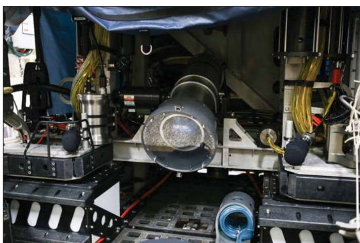
LEFT: Commander Mark Wetzler, commanding officer of the Okeanos Explorer, shows off a bit of the technology that powers the ship's dedicated Deep Discoverer remotely operated vehicle; at a cost of $5, the ROV was built in house at NOAA, lives permanently on the Okeanos and can dive down to a depth of 6,000 meters—lower than the elevation difference of Mount Kilimanjaro. RIGHT: D2's high precision cameras are the best in the field, in terms of oceanic exploration and research, Wetzler says.
