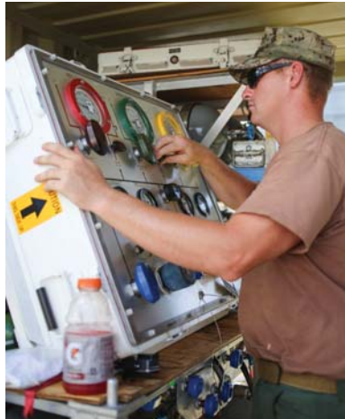
sw2 David Miller controls the delivery of gases to the divers below using what Bravo calls the surface-supplied system.
