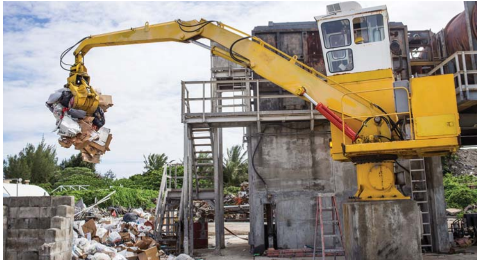
Solid Waste employee Rodderick Capella hoists a load of trash with a newly-overhauled grappler crane at the Kwajalein landfill April 3. Part of a 10-month, multi-department repair project, the cranes and refurbished incinerators are in full use, eating away at trash that had been piling up on the Solid Waste grounds for months.
