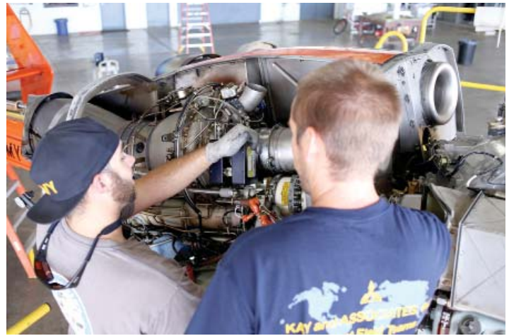
Josh Weiner, left, and Jobe Bell install a new alternator, or generator, into the engine compartment of the aircraft at the Helicopter Maintenance Facility.
