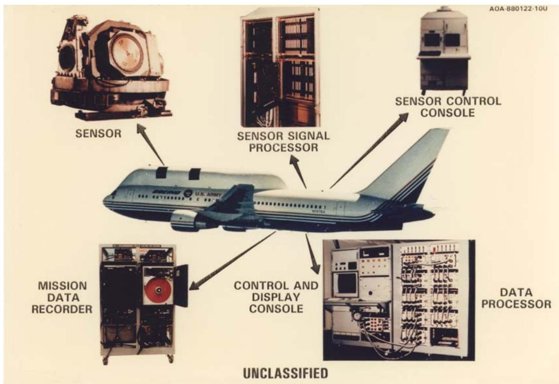
*Fig. 3-25. The Airborne Surveillance Testbed, an airborne system with its heat detecting telescope, remains an important asset to Army data collection efforts. This diagram illustrates the various components of the AST system.*
