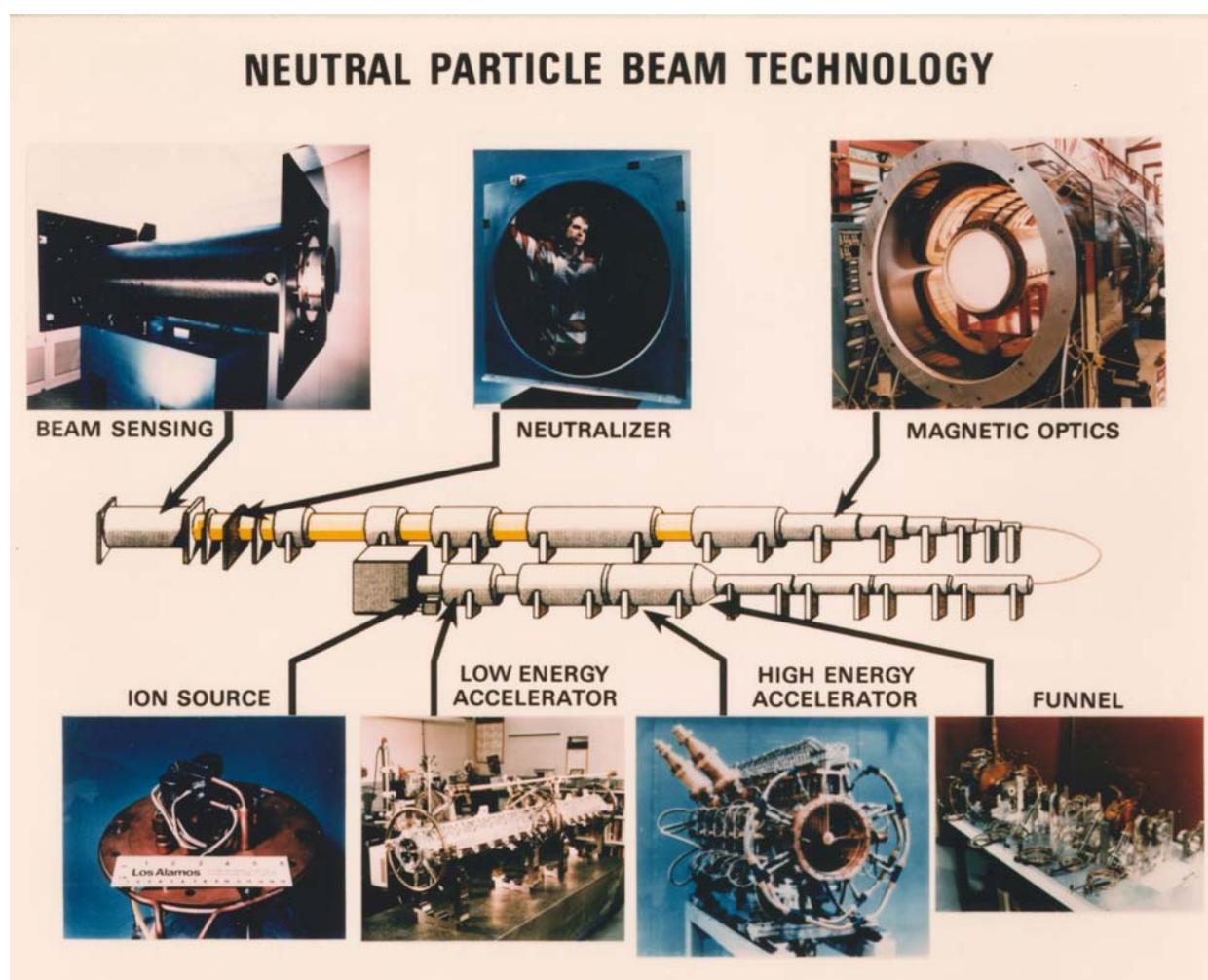
*Fig. 3-20 and 3-21. By 1993, many of the Neutral Particle Beam technologies had reached maturity. The diagram above shows the elements of an NPB and their place in the finished product. A deployed NPB (depicted on the facing page) would be a space-based system which could shoot hydrogen molecules at about 60,000 kilometers per second.*
