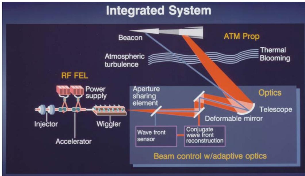
*Fig. 3-18 and 3-19. These artists' concepts illustrate the proposed missions of the Ground-Based Laser. The first shows the Integrated System of the ground-based free electron laser. The second illustrates the system components for a theoretical ground-based laser anti-satellite system.*
