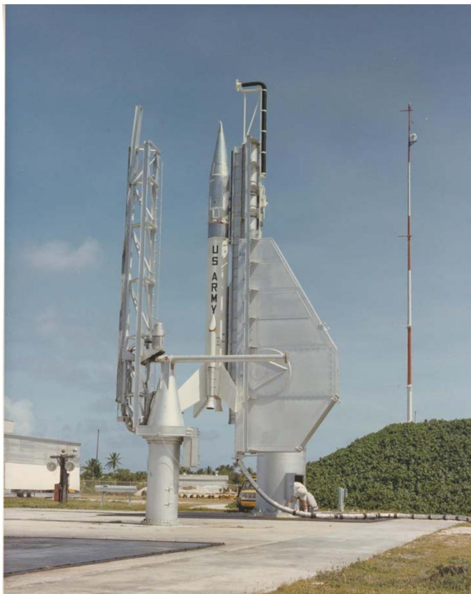
*Fig. 3-4. The Designating Optical Tracker (DOT) enjoyed a perfect test record and demonstrated the viability of the onboard infrared optics technology. The DOT on its launch pad at the Kwajalein Missile Range.*
