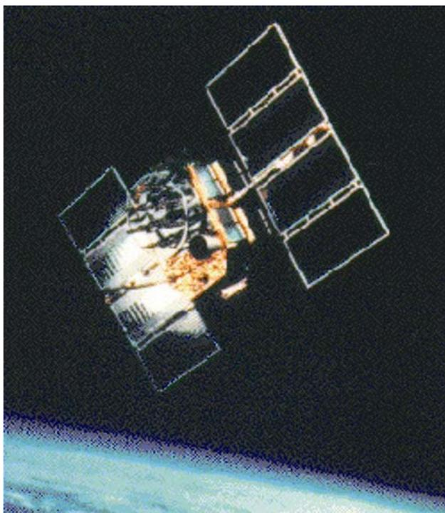
*Fig. 3-32. Artist's drawing of a Global Positioning System satellite.*
