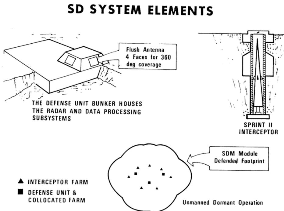
*Fig. 3-1. The artist's drawing illustrates the system elements of the Site Defense concept and its proposed deployment within the defense unit.*
