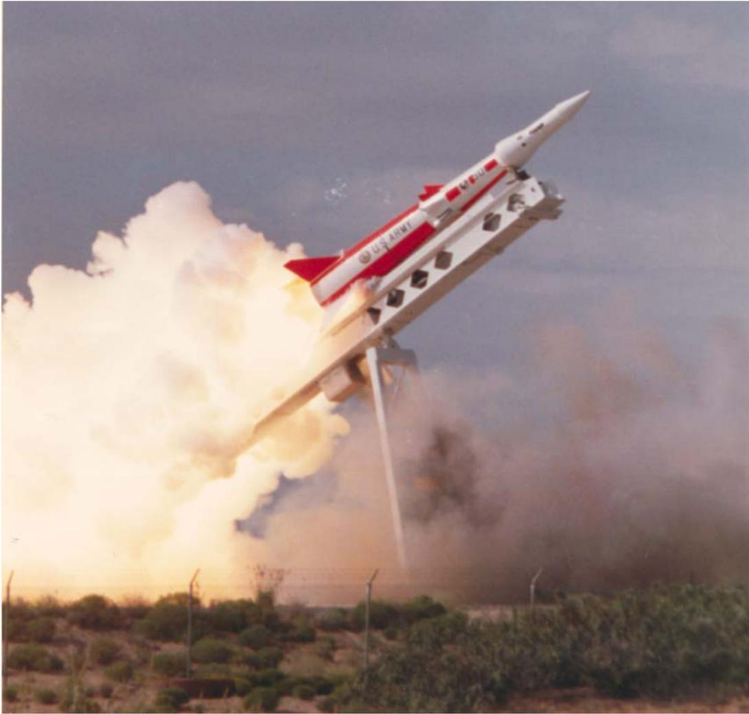
*Fig. 3-29. The rail-launched High Endoatmospheric Defense Interceptor missile achieved a successful intercept in this Kinetic Intercept Technology Experiment 2A conducted on 25 August 1992.*
