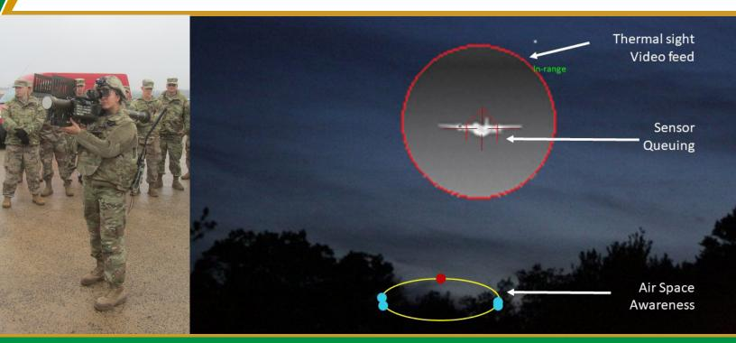
ETAK provides day/night and degraded visual environment target acquisition and tracking for man portable systems
