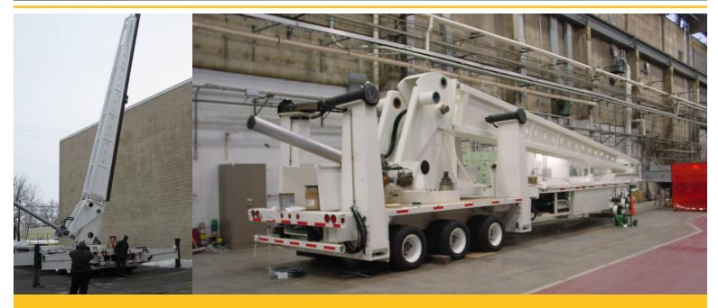
The Test Directorate developed two launchers capable of launching 25,000-pounds static load rockets
