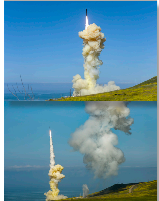
Two Ground-based Interceptors are launched from Vandenberg Space Force Base March 25, 2019, in the first-ever salvo flight test of the GMD system. The GBIs intercepted a threat-representative ICBM target launched from the Marshall Islands. (Missile Defense Agency)
